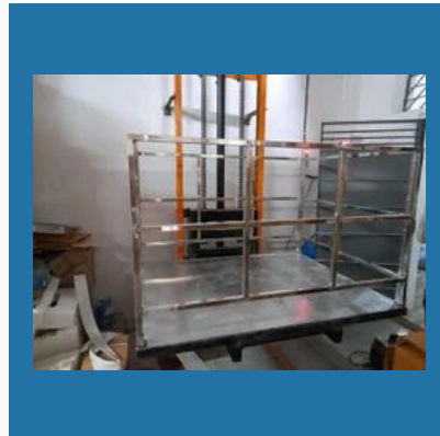
Mezzanine Floor Goods Lift
